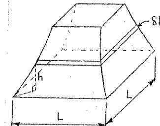
A stone building of height  $H$  metres has the shape of a flat topped square 'pyramid' with curved sides as shown in the figure. The cross-section at height  $h$  metres is a square with sides parallel to the sides of the base and of length  $l$ ,  $l = \frac{L}{\sqrt{h+1}}$  where  $L$  is the side length of the square base in metres.
